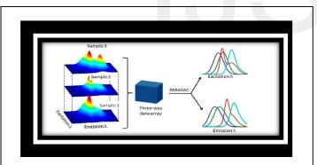
Fig 3. Schematic representation of the PARAFAC operation ,which builds a three way data array with the different data matrices, and then decomposes the array in both instrumental data modes (in this case excitation and emission fluorescence loadings as a function of wavelength,.sample scores are also produced, containing information relative to constituent concentrations.
